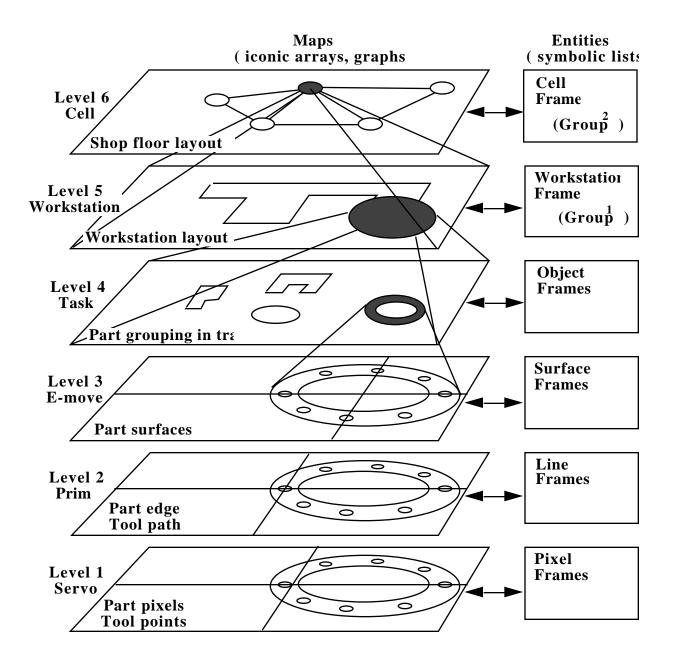
Figure 10. Map-entity relationships in a world model for manufacturing. The world model provides processes by which symbolic entity frames can be transformed into maps, and vice versa.
