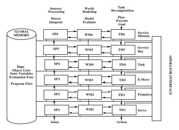
Figure 2. The NASREM (RCS-3) control system architecture.
