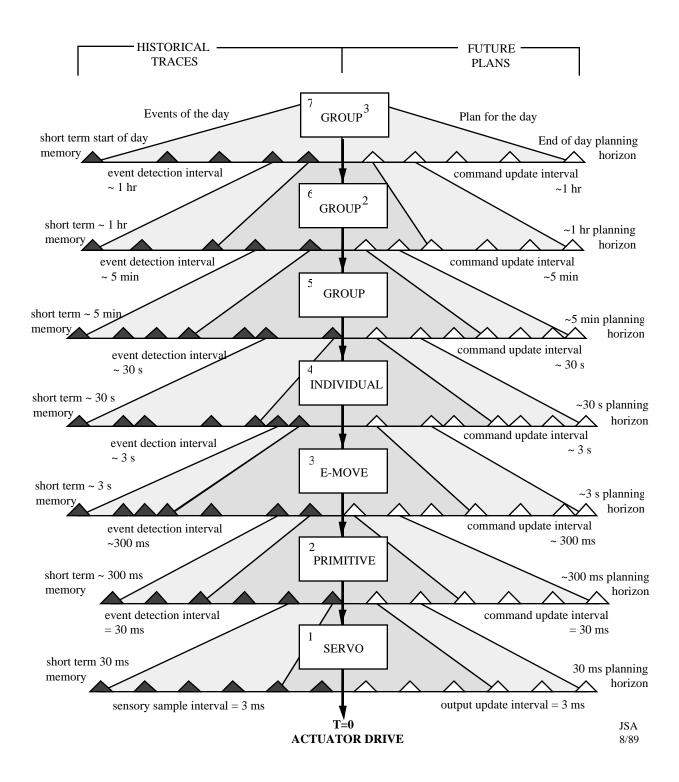
Figure 5. Atiming diagram illustrating the temporal flow of activity in the task decomposition and sensory processing systems.
