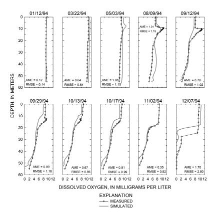
Figure 12. Relation between measured and simulated dissolved-oxygen concentrations in the water column near the Beaver Lake dam, January through December 1994.
