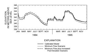
**Figure 18.** Simulated surface elevations resulting from additional minimum flow with and without increasing pool elevation.
