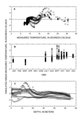
Figure 11. Relation of difference between measured and simulated water temperatures near Beaver Lake dam to (a) measured water temperature, (B) date, and (C) water depth, January through December 1995.
