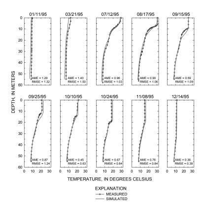
Figure 10. Relation between measured and simulated water temperatures in the water column near the Beaver Lake dam, January through December 1995.
