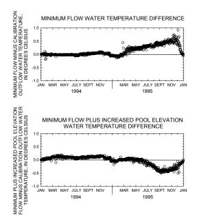
**Figure 21.** Simulated water temperature difference between calibrated base condition and additional minimum flow scenarios.
