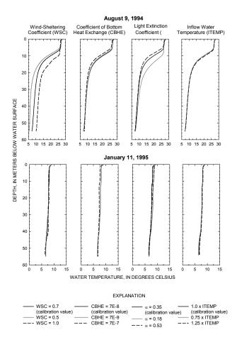
**Figure 16.** Vertical temperature distributions near the Beaver Lake dam on August 9, 1994 (top) and January 11, 1995 (bottom), showing calibrated model profiles and profiles as a result of differing model parameters.
