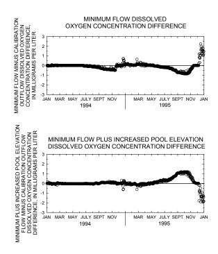
**Figure 23.** Simulated dissolved-oxygen concentration differences between calibrated base condition and additional minimum flow scenarios.
