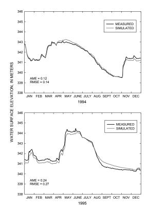
**Figure 7.** Measured and simulated water-surface elevation near the Beaver Lake dam, January through December 1994 and January through December 1995.
