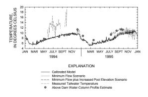
Figure 20. Simulated water temperatures in Beaver Lake outflows and measured in the tailwater.
