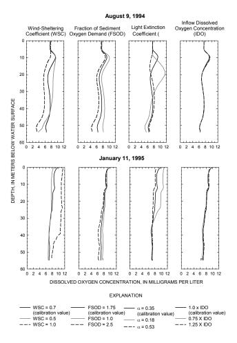
**Figure 17.** Vertical dissolved-oxygen concentration distributions near the Beaver Lake dam on August 9, 1994 (top) and January 11, 1995 (bottom), showing calibrated model profiles and profiles as a result of differing model parameters.
