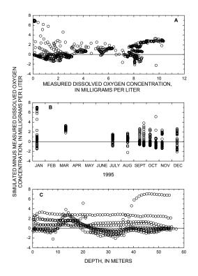
**Figure 15.** Relation of difference between measured and simulated dissolved-oxygen concentrations near Beaver Lake dam to (A) measured dissolved-oxygen concentrations, (B) date, and (C) water depth, January through December 1995.
