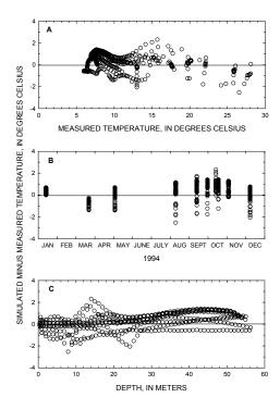
**Figure 9.** Relation of difference between measured and simulated water temperatures at Beaver Lake dam to (A) measured water temperature, (B) data, and (C) water depth, January through December 1994.
