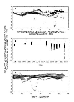
**Figure 13.** Relation of difference between measured and simulated dissolved-oxygen concentrations near Beaver Lake dam to (A) measured dissolved-oxygen concentrations, (B) date, and (C) water depth, January through December 1994
