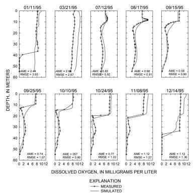
Figure 14. Relation between measured and simulated dissolved-oxygen concentrations in the water column near the Beaver Lake dam, January through December 1995.
