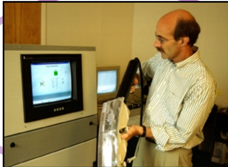
SpectraCode's RP-1 system is being used to identify the plastic backing on an automobile headlight. This technology can identify plastics so they can be sorted for recycling, including plastics that currently are impossible or difficult to sort.
