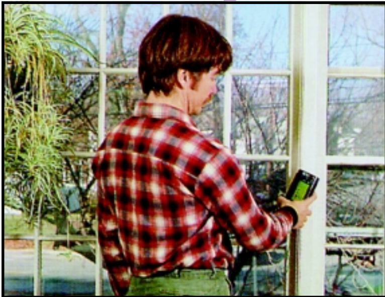
NITON's XL-309 Dual Detector Lead Paint Analyzer fits in window wells, mullions, and decorative molding with a 1 cm x 2 cm window located at the front edge of the XL.
