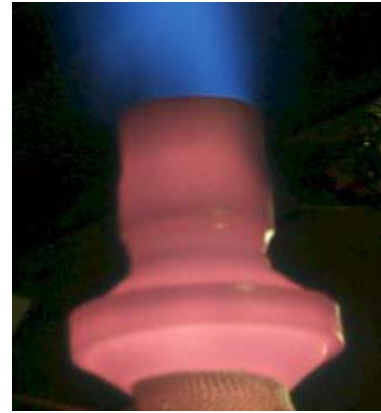
PCI's Microlith® automotive preconverter undergoing a hot vibration test (100 Hz, 28 g, at 950°C for 150 hours).
