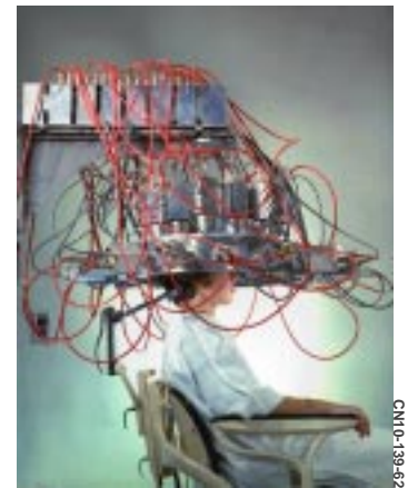
Rankowitz and colleagues designed and built the BNL "hair dryer," a pioneering device in the early days of positron emission tomography (PET) technology.
