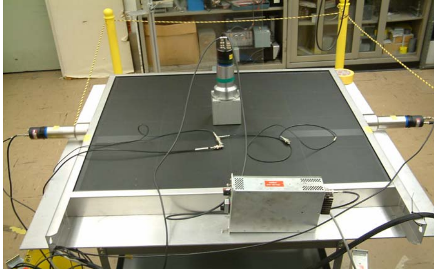
Figure 2. 1x1 meter plastic scintillator detector with a 3.75x3.75 inch plastic scintillator detector resting on top.
