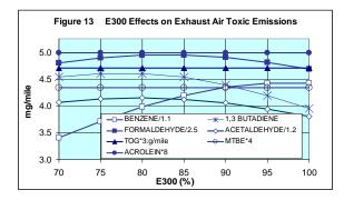
Formaldehyde, acetaldehyde and 1,3 butadiene exhaust emissions increase as E300 increases from 70.0% to 80.0%. Between 80.0% and 100.0%, the emission factors for these three compounds decrease as E300 increases.
