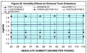
Humidity impacts on air toxic emissions are shown in Fig. 29. As humidity increases, all exhaust emissions including all air toxic compounds, MTBE and TOG increase at a similar factor. Humidity has no effect on evaporative emissions.
