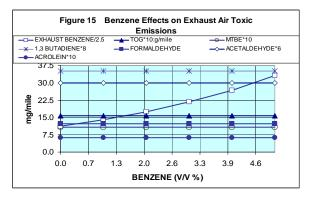
linearly (Fig. 15). This same linear response is also observed with the evaporative benzene emission factors. No other air toxic compound emission factors are affected by benzene content.
