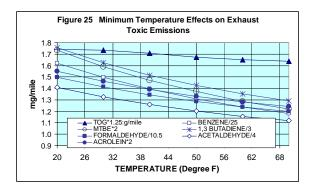
As indicated in Fig. 25, all exhaust air toxic compounds and TOG emissions increase as daily minimum temperature decreases. All emission factors are virtually parallel to each other. As the daily maximum temperature increases, all exhaust emissions increase (Fig. 26). However, all air toxic compound emissions are at a much lower rate than the TOG emission factor.
