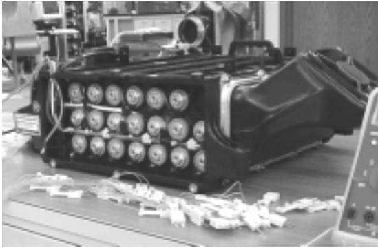
Figure 1 – Honda Insight Battery Pack
