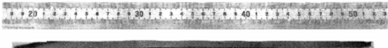
Fig. 1.24. First demonstration of an ~30-cm-long CeO 2 -buffered Ni substrate using a rotating cylinder in the e-beam evaporator. Ni substrate = 5 mil; CeO 2 thickness = 1,000 Å.
