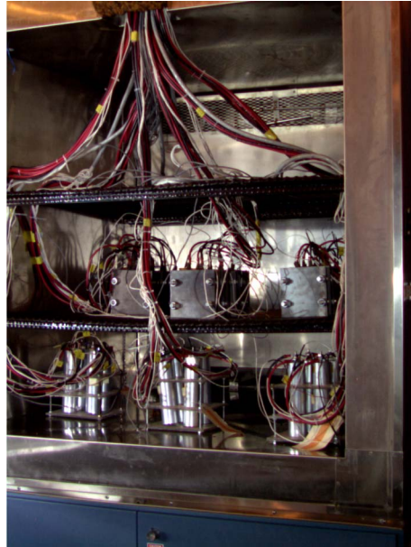
Figure 1.—Saft (lower) and Lithion (upper) cells configured in packs in test chamber.
