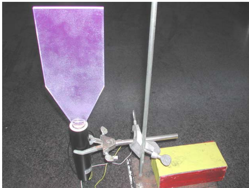
Figure 13: Scintillator bonding with the end mount photomultiplier undisturbed for 24-48 hours.
