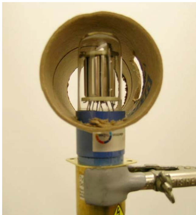
Figure 18: Side mount photomultiplier in cardboard tubing.
