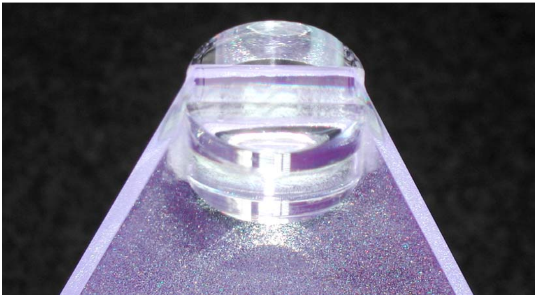
Figure 9: Polished surface of scintillator.
