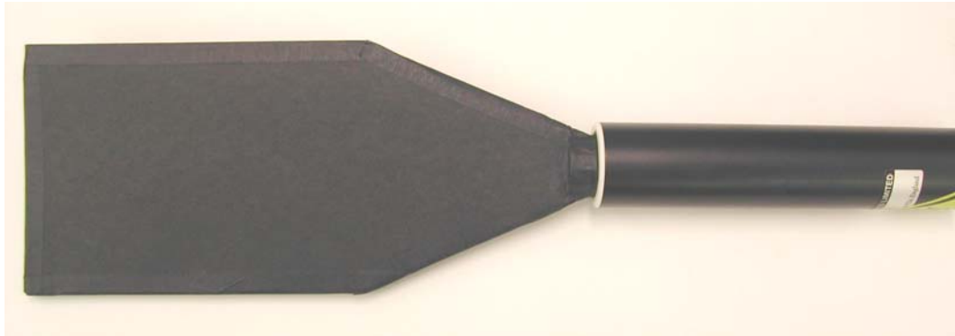
Figure 14: Finished scintillator attached to end mount photomultiplier.
