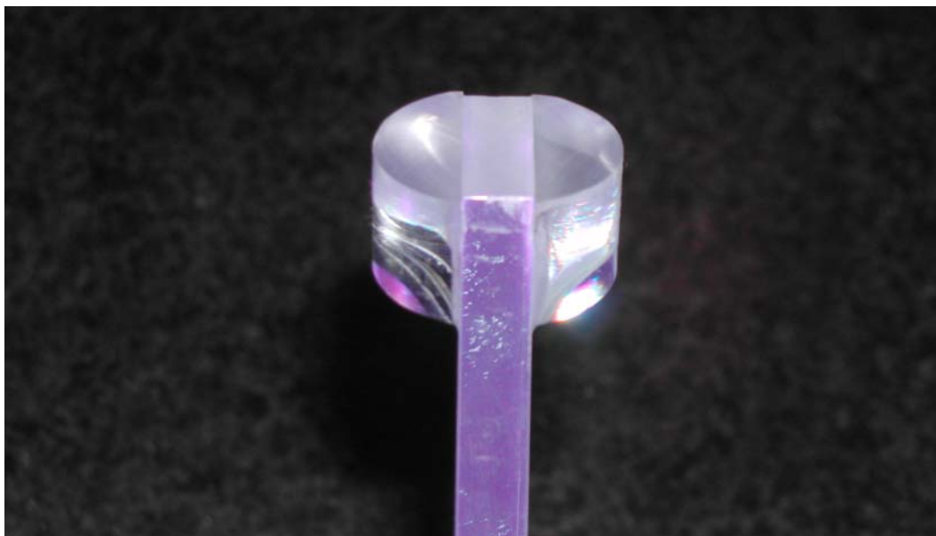
Figure 4: Lucite cookies (half cylinders) attached to 3/4-inch end of scintillator (center strip).
