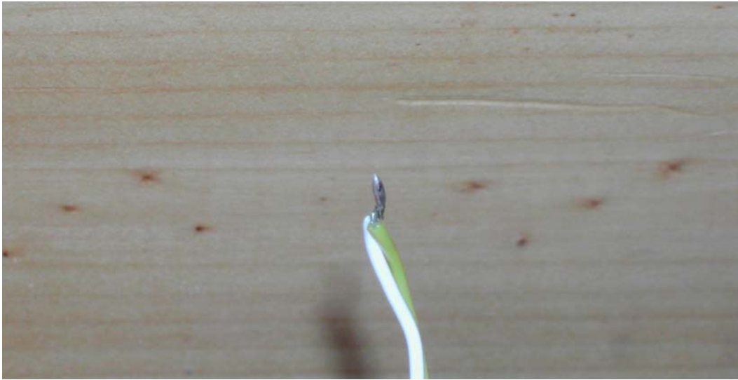
Figure 31: Gain wire shorted.
