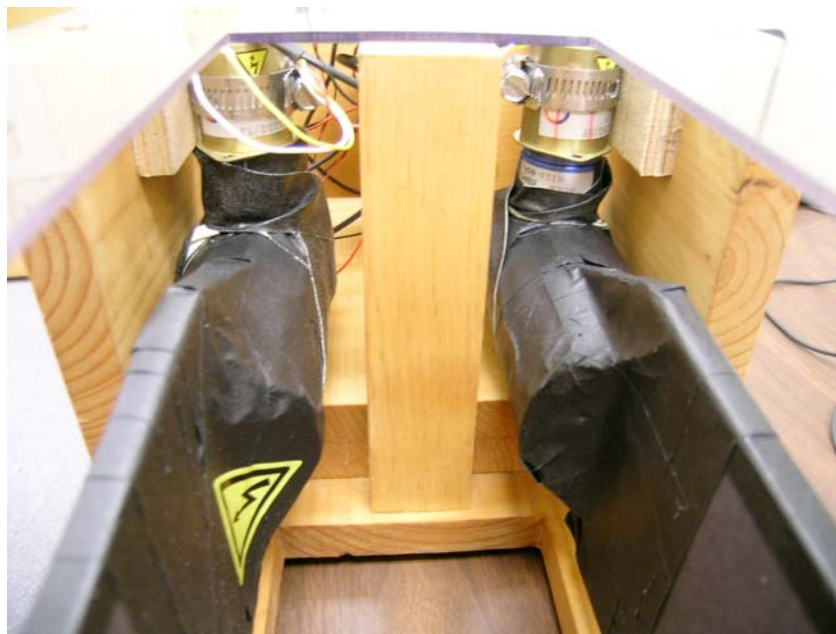
Figure 19: Side mount photomultipliers attached to scintillators.
