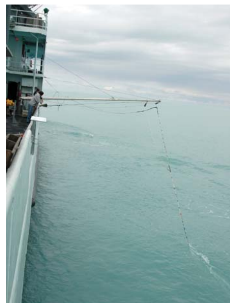
Ken Bruland's "fish" surface-water-sampling system collecting surface-water samples from the sediment-laden Alaska Coastal Current in the Gulf of Alaska on the research vessel Thomas G. Thompson . Photograph by Ken Bruland .
