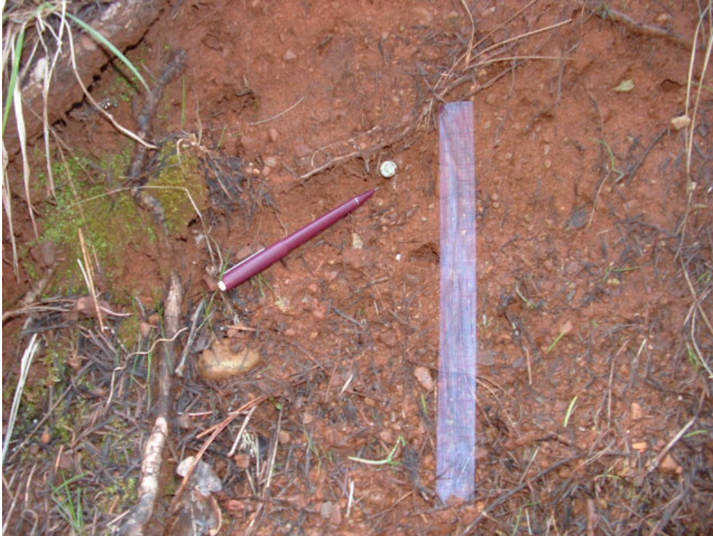
Figure 24. Example of erosion pin installed in road cutbank. Pencil points to top of erosion pin exposed following winter storms.
