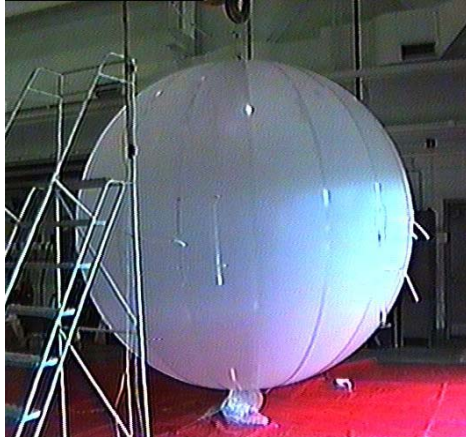
Spherical balloon would have much higher stresses
