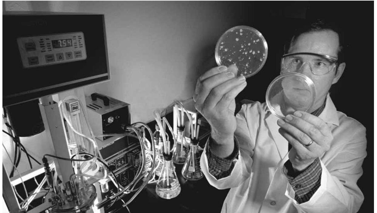
IN THIS 1999 LAB NEWS PHOTO, Mark Tucker (6327) examines two petri dishes: one with a simulant of anthrax growing in it (left), the other treated with the decontaminating foam developed at Sandia (right). The nonhazardous foam begins neutralizing both chemical and biological agents in minutes. Next to Mark is a flask containing about a liter of bacillus globigii , the nontoxic simulant of anthrax used in experiments at Sandia. (Photo by Randy Montoya)
