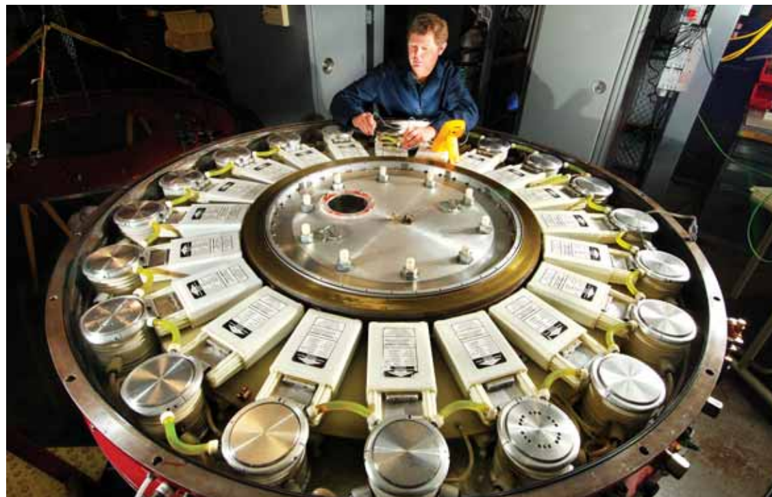
AREA 51? NO, AREA 4 — Bill Fowler checks out a linear transformer driver device from Siberia that could replace the arcs-and-sparks generation of the current Z machine. The row of switches (circular devices) are connected to capacitors (rectangular objects). The tubes contain liquid resistors. (Photo by Randy Montoya)
