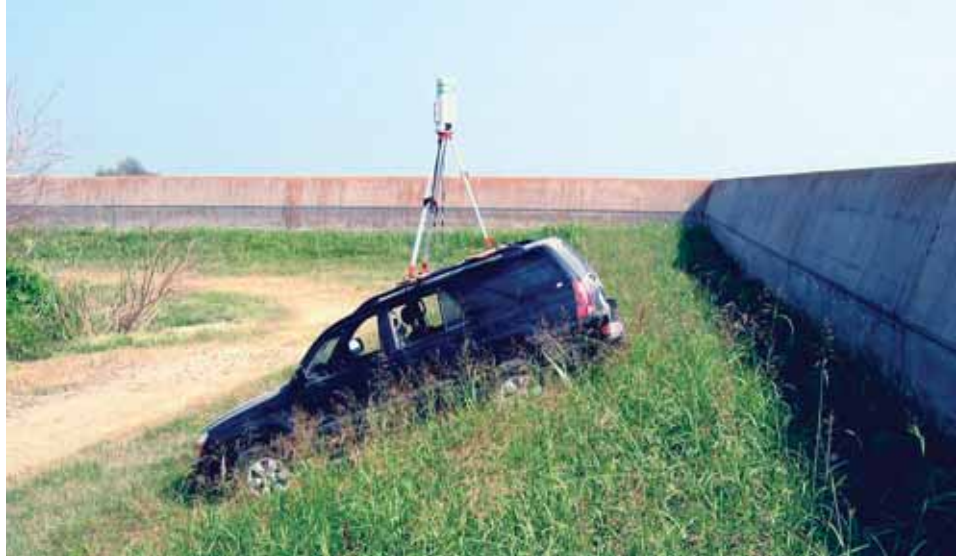
Lidar unit and tripod mounted to the roof of Kayen and Collins’ field vehicle. The fixed roof base allowed for leveling of the tripod and lidar instrument on sloping ground. Here the instrument is scanning scour at the base of intact floodwall at an Entergy New Orleans plant in east New Orleans (survey site 10). Photograph by Robert Kayen.
