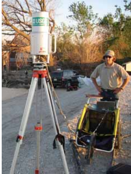
Tripod-mounted lidar (light detection and ranging) unit at the 17th Street Canal breach (survey site 1). Brian Collins mans a pushcart containing a laptop computer and other electronics connected to the lidar unit. Photograph by Robert Kayen .
