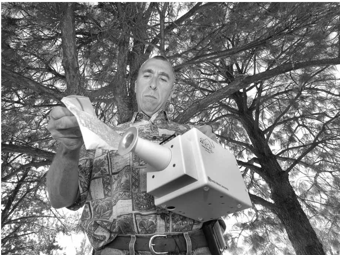
DRUG SNIFFER — Dave Hannum demonstrates use of the Hound system, which includes preconcentration technology developed at Sandia, on a bag of white powder. The hand-held system, originally developed for explosives detection, also can detect and identify illegal drugs. The South Texas Specialized Crimes and Narcotics Task Force is using a Sandia prototype to catch drug smugglers. (Photo by Randy Montoya)
