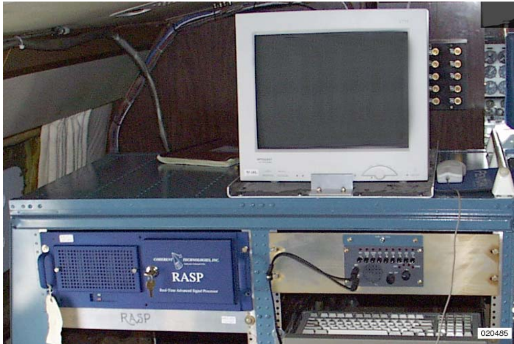
Figure 7. Flight-qualified real-time advanced signal processor (RASP) and display.
