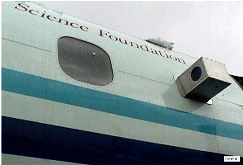
Figure 22. Folding mirror housing on the Electra test bed aircraft.
