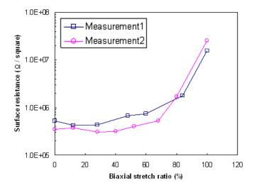
**FIGURE 9:** Surface resistance of PAni-EVAelectrodes as a function biaxial stretch ratio.
