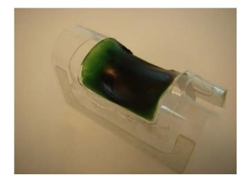
**FIGURE 10:** Soft frame actuator prototype with PAni-elastomer electrodes.
