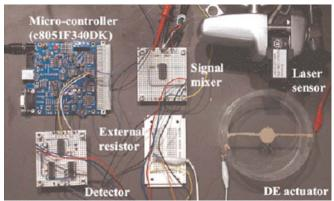
**FIGURE 2:** Dielectric elastomer (DE) actuator and sensor.
