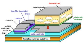
**FIGURE 7**: Concept of the "ferroelectret fieldeffect transistor". The voltage generated by the ferroelectret upon touching the element, or by means of acoustical waves controls the current through the flexible field-effect transistor.
