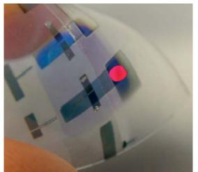
**FIGURE 8:** Operation of a flexible optothemal switch, based on pyroelectric copolymers of vinylidene fluoride and trifluoroethylene and - voltage organic field-effect transistors.
