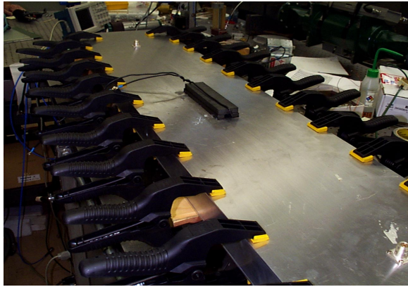
Figure 5. Waveguide is shown with ferrite magnets with two coax-to-waveguide transitions and clamps.
