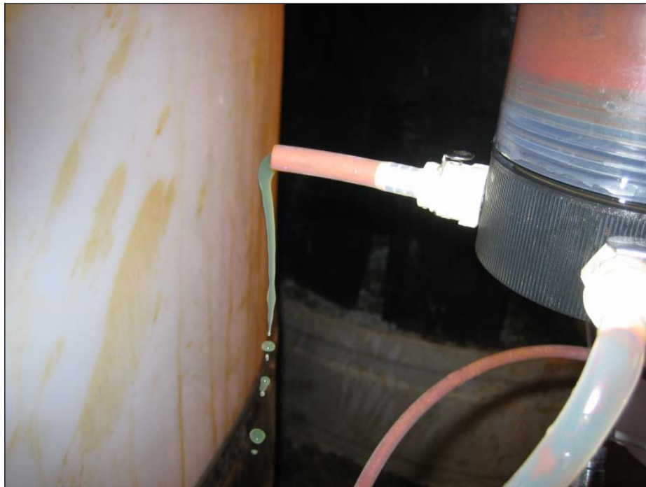
Figure 40. Water from the third step, iron build up on the flow cell
