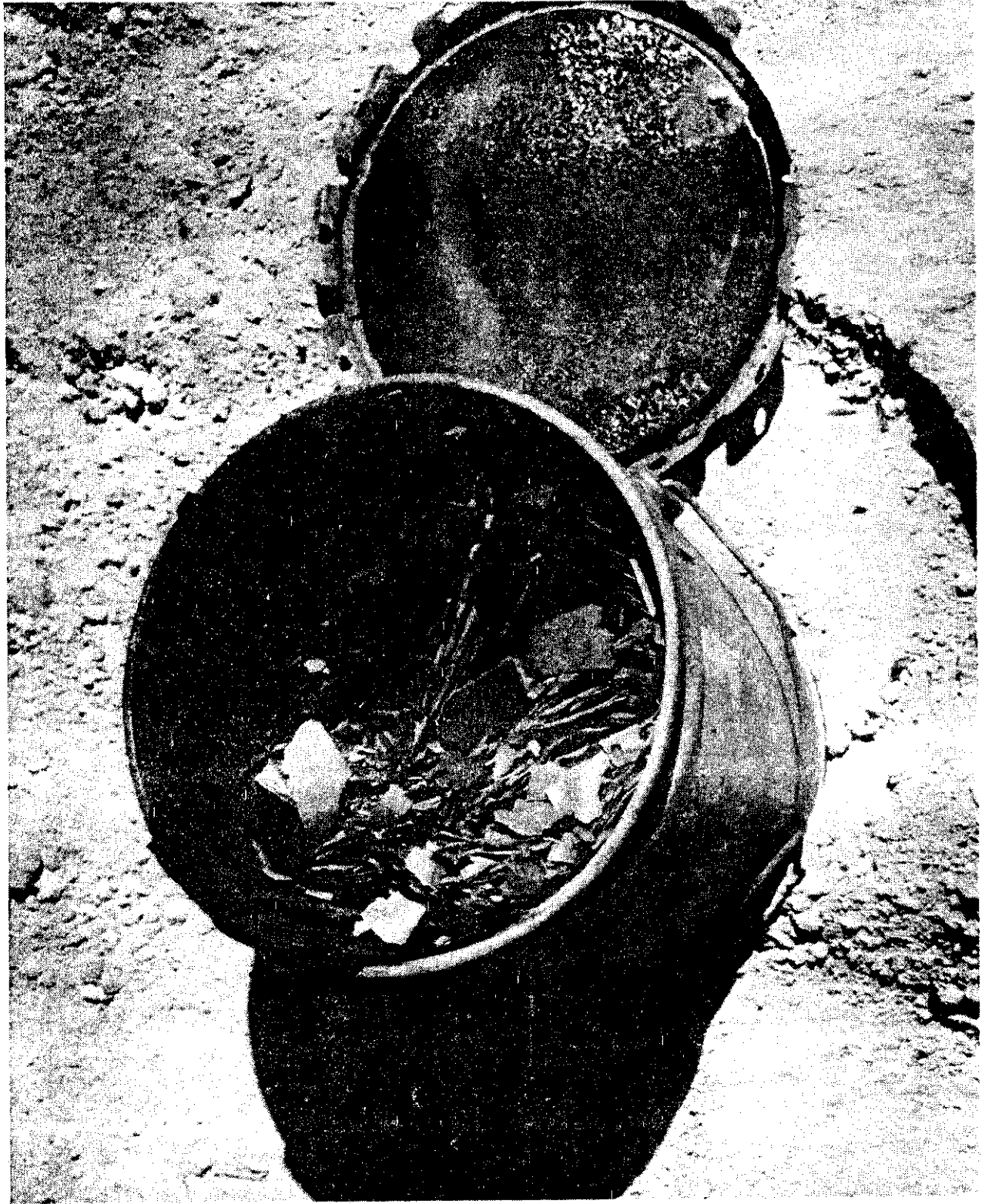
Figure 102. Carbonization of paper outside of vitrification zone for Test Pit 2.
