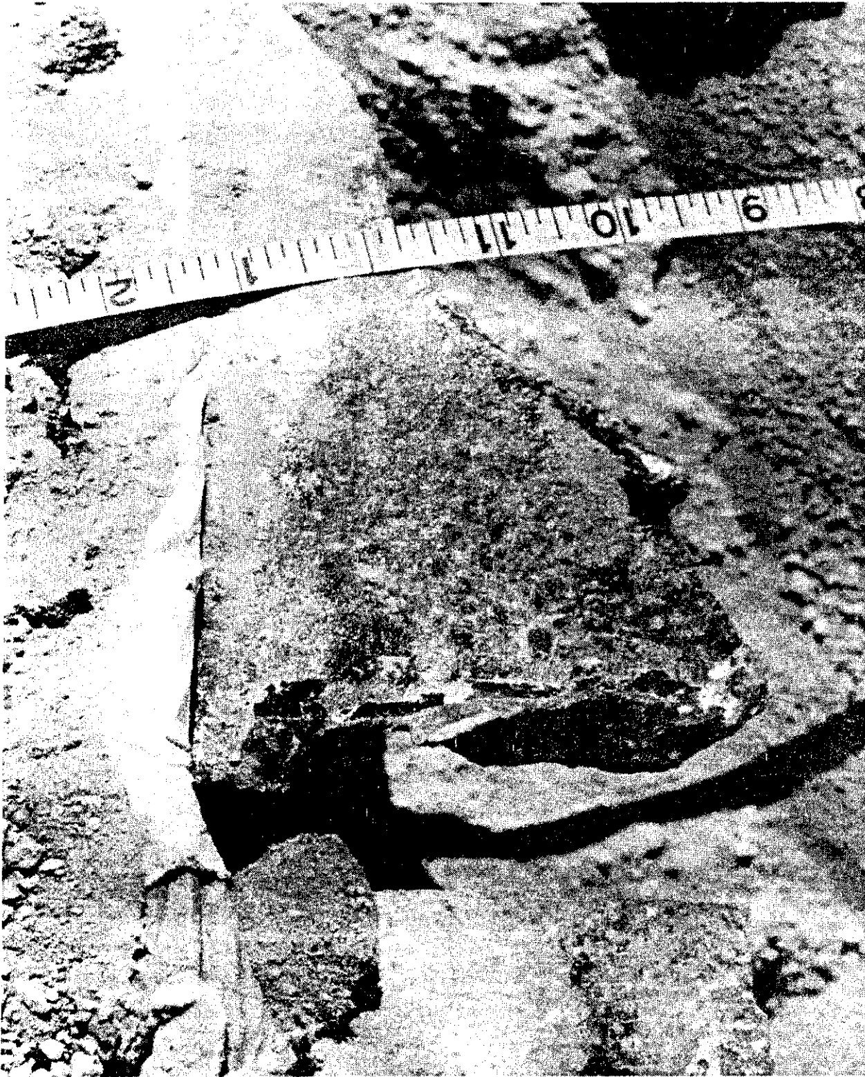
Figure 103. Edge effect showing molten steel near cardboard in Test Pit 2.
