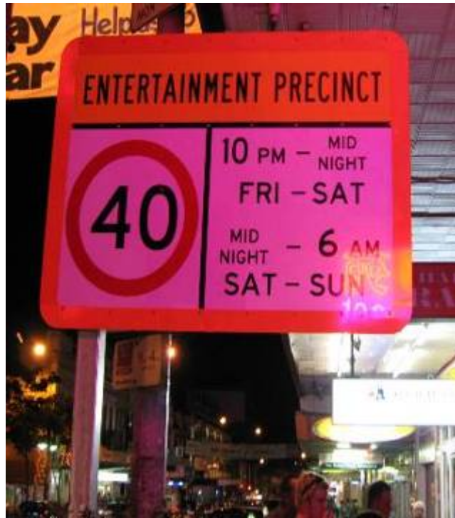
Figure 3. Reduced speed zone in high-pedestrian traffic area in Brisbane, Australia. Similar speed zones exist in other Australian states for shopping districts and school zones.
