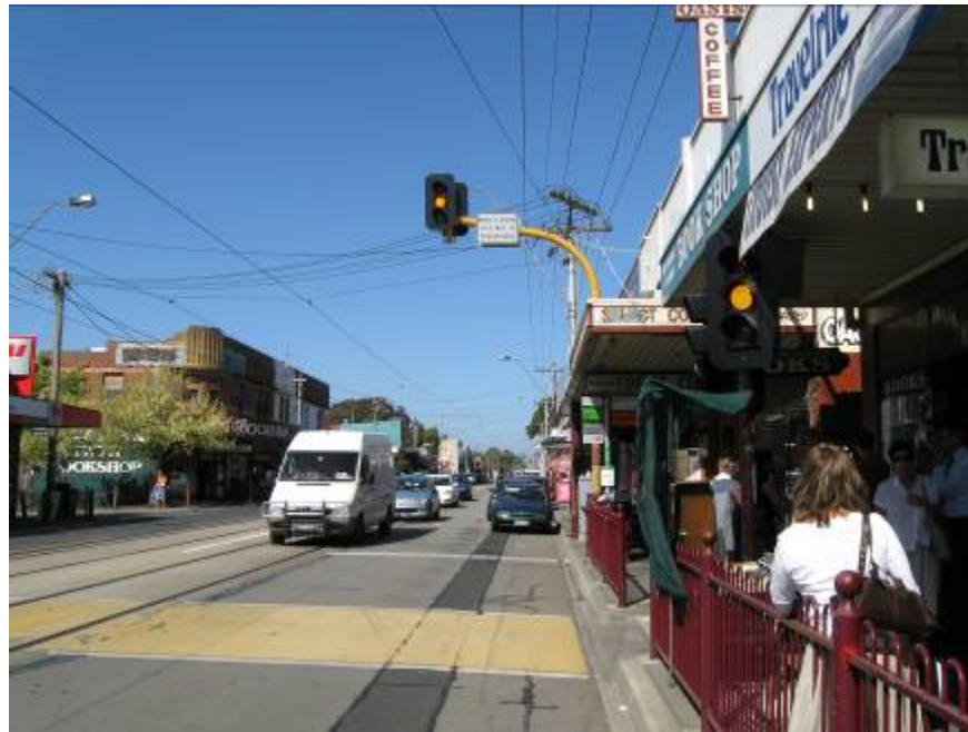
Figure 8. Mid-block pedestrian actuated crossing with pedestrian fencing in Melbourne, Australia.
