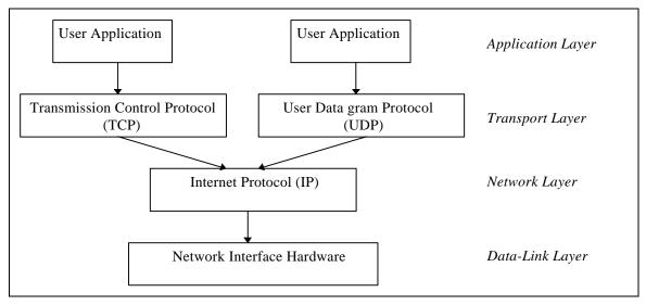
Figure 5: UDP placement in the four Layer OSI Protocol Model.
