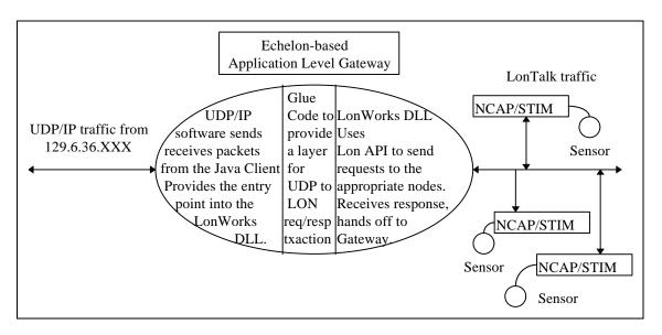
Figure 4: Example of a possible Echelon Application-Level Gateway.
