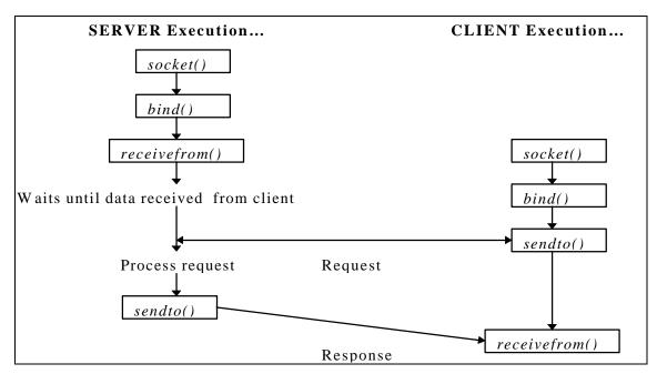
Figure 7: Server startup using Socket calls in a connectionless Protocol mode.
