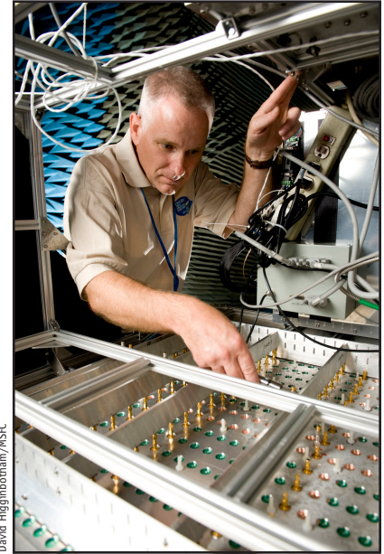
Mark James, Marshall's Hurricane Imaging Radiometer lead engineer, adjusts components on the rear of the HIRAD antenna before a test run.
