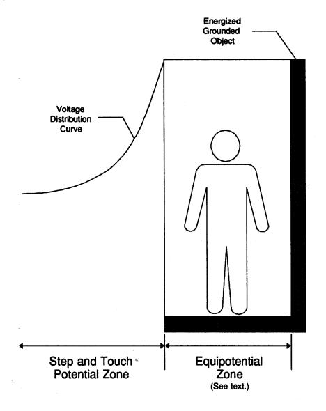
Figure 3 - Protection from Ground-Potential Gradients
