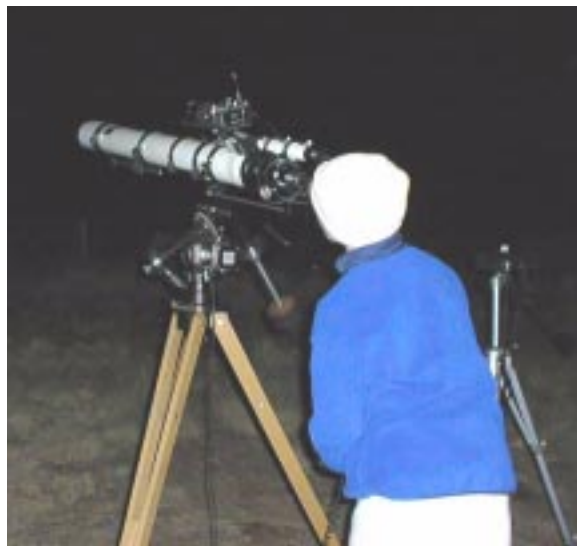
Figure 1: My camera is mounted piggy-back on the large telescope, which I used for guiding on a star while taking pictures for 1 minute to 10 minute exposure times, depending on the film speed I was using, or whether clouds or the neighbor's lights were bad.
