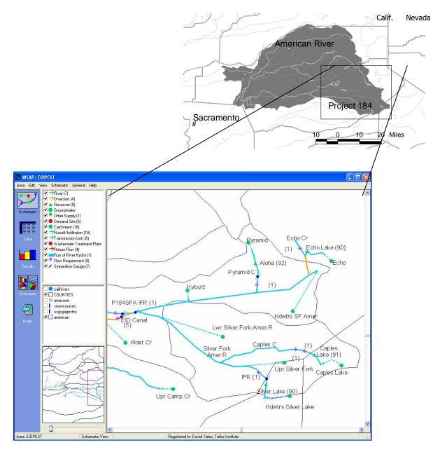
**Figure 2.** EID's Project 184 system as represented in the WEAP DSS. The 10 dots and their connecting dotted lines represent individual sub-catchments (Pyramid, Echo, Headwaters South Fork American, etc.). The four triangles are the reservoirs (Silver, Caples, Aloha and Echo), while the hatched circles are in-stream flow requirements.
