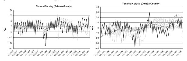
Figure 5.7. Net annual groundwater flux to (positive) and from (negative) the surface water system of the Sacramento Valley Rivers.
