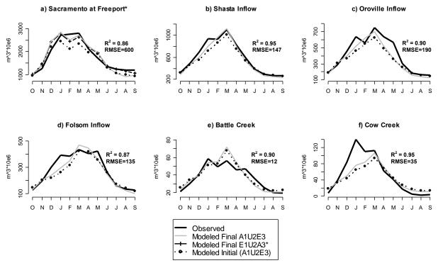
Figure 5.2. Observed and modeled average monthly streamflow for a) The Sacramento at Freeport, (plot includes average flows based on both the A1U2E3 and the E1U2A3<sup>\*</sup> scenarios); the inflows to the three major reservoirs, b) the Pit and Upper Sacramento Rivers; c) the Feather River; and d) the American River; and two minor tributaries including e) Battle Creek and f) Cow Creek. Inset includes correlation coefficient ( $R^2$ ) and the root mean square error (RMSE, \*10E6 m3).
