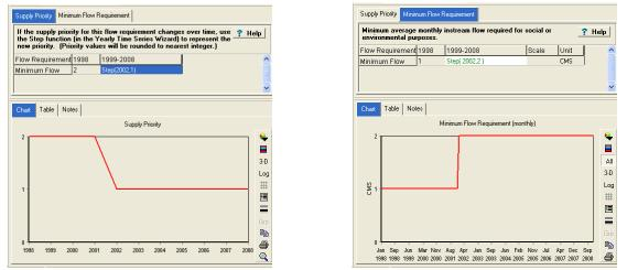
Figure 4.7. WEAP21's GUI for specifying instream flow requirements. The left panel shows the supply priority of instream flow, while the right panel is the actual instream flow requirement in m<sup>3</sup>/s. that abruptly change over time as a result of regulatory requirement.
