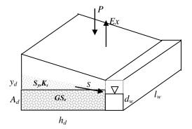
Figure 4.5. Schematic of the stylized groundwater system, and its associated variables.
