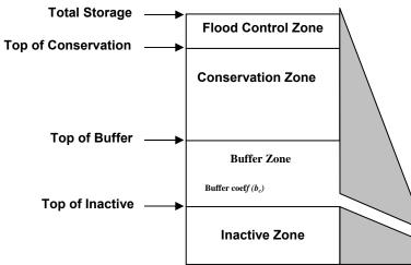
Figure 4.8. The different reservoir storage volumes used to describe reservoir operating policies.
