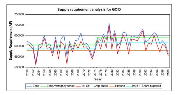
Figure 6.29. Changes in supply requirement associated with improvements in irrigation technology and dynamic cropping patterns—GCID
