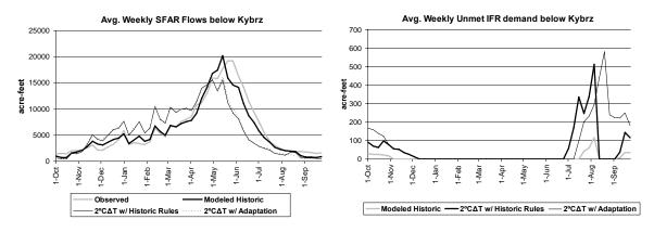
**Figure 3.** Observed and simulated streamflow values for the South Fork American River below Kyburz (left) and the unmet portion of the new FERC IFR for the South Fork American River below Kyburz (right)
