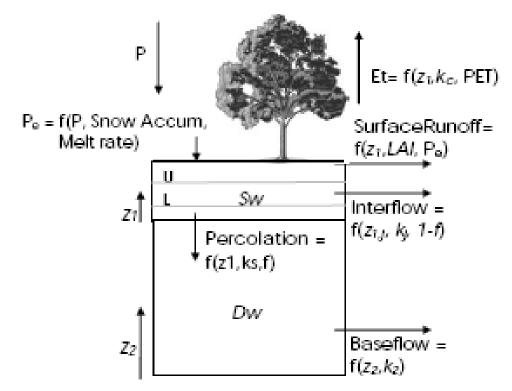
Figure 4.4. Schematic of the two-layer soil moisture store, showing the different hydrologic inputs and outputs for a given land cover or crop type, j
