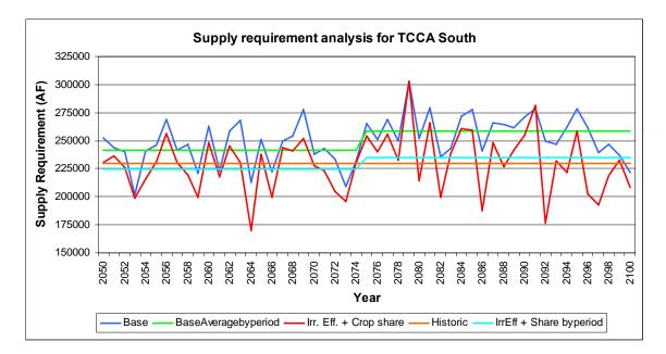
Figure 6.28. Changes in supply requirement associated with improvements in irrigation technology and dynamic cropping patterns—TCCA South
