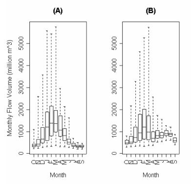
Figure 2.4: Monthly Flow Volumes in the Sacramento River below Shasta Dam as (A) an Estimate of the Full Natural Flow and (B) the Observed Flow
