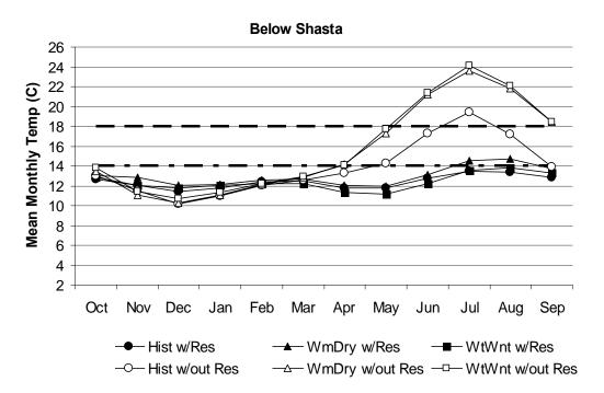
Figure 7.6. Modeled historic and future (average for "2060 to 2100") mean monthly water temperatures in the Sacramento River near Redding. The top, horizontal dashed line represent the 18°C for juvenile emigration and the bottom, 14°C spawning and rearing threshold conditions.
