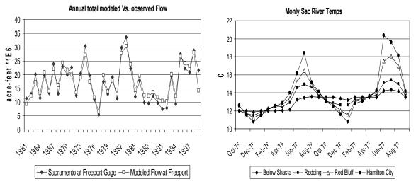
Figure 7.5. Time series of historic and simulated river flows and simulated river temperatures along select reaches.
