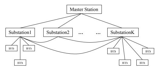
Figure 1: A Model SCADA Network
