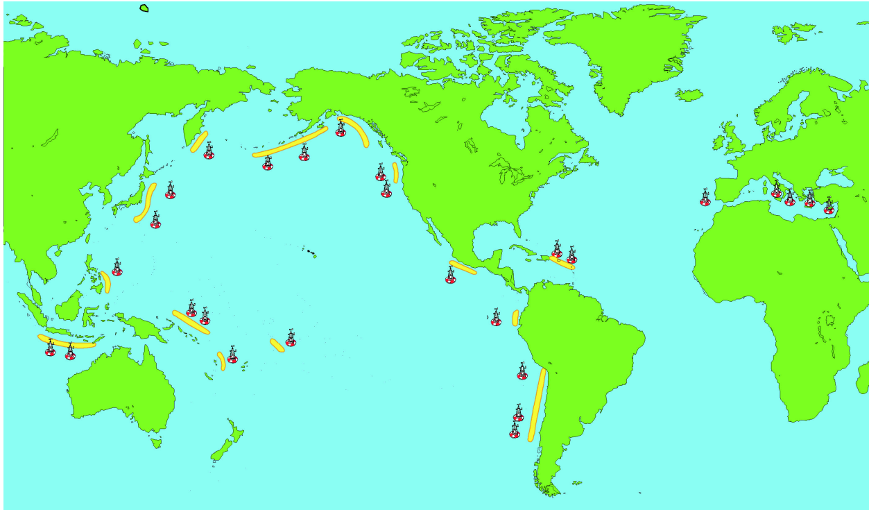
Figure 8: Preliminary siting of worldwide tsunami detectors. Yellow bands are seismically active areas that have generated tsunamis in the past.
