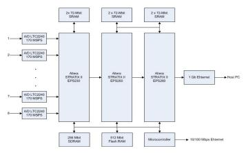
Fig. 4 DBSAR processor diagram showing main components.
