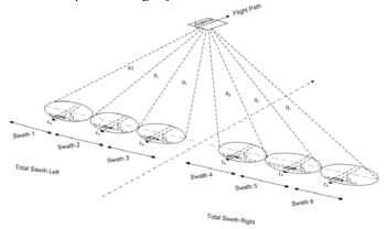
Fig. 5 Digital beamforming SAR operational mode
