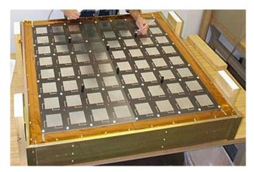
Fig. 2 Dual-polarization micro-strip patch antenna
