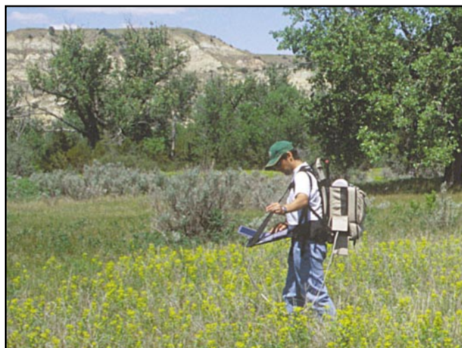
FIGURE 8. Raymond Kokaly (USGS) measures the reflectance of vegetation using a field spectrometer (Photo courtesy of R. Kokaly)
