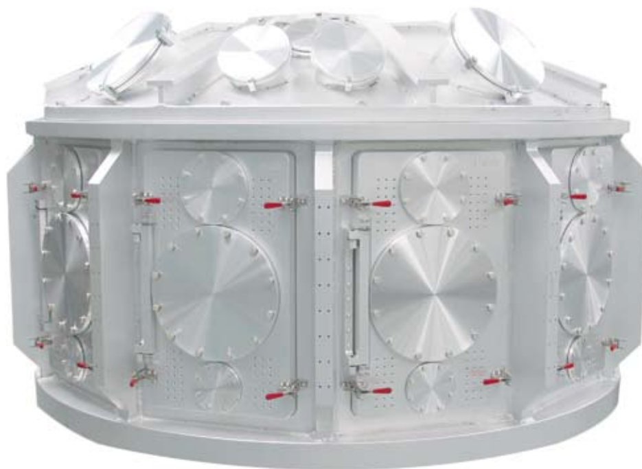
Titan’s long-pulse beam can be directed into the 2.5-meter-diameter target chamber through different ports. The short-pulse beam is directed through a dedicated port.
