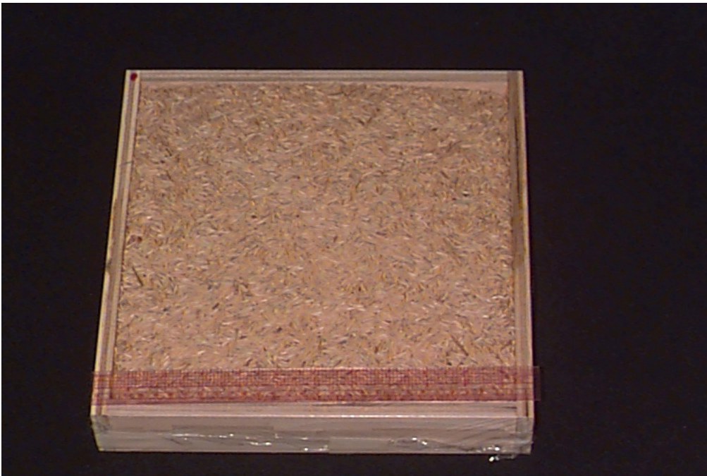
Figure 1. Photograph of Rice Hull Thermal Test Specimen
