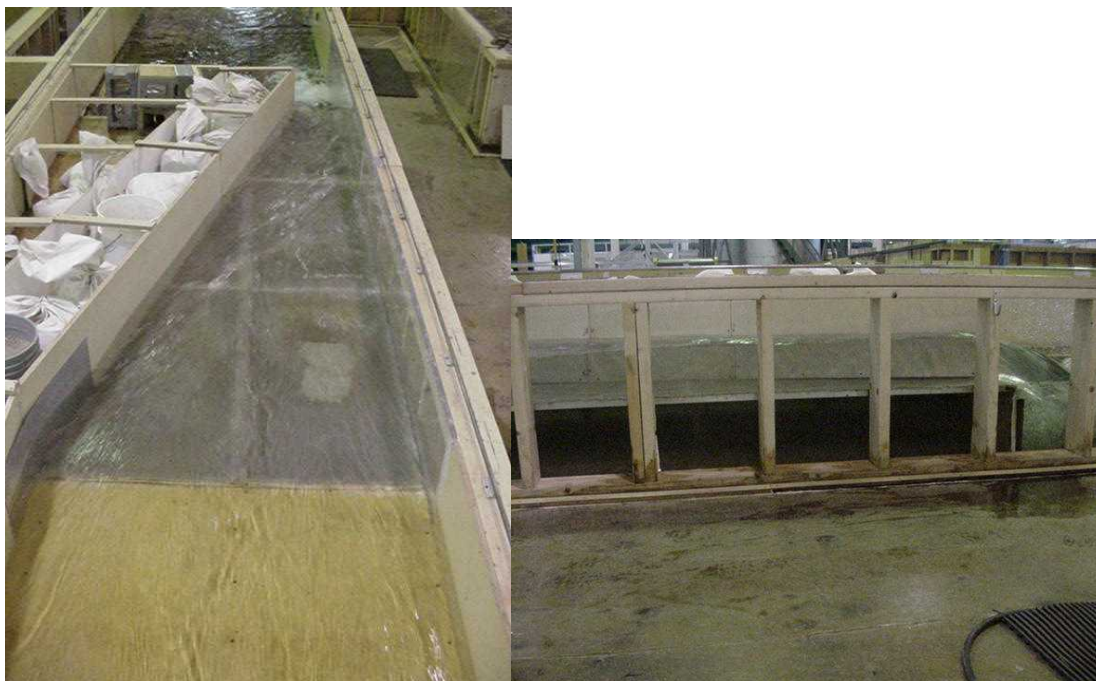
Figure 28.—Test 18. Critical flow at the downstream end of the screen with Q_c = 9 \text{ ft}^3/\text{s} and Q_d/Q_c = 74 percent. Flow depth of 0.5 ft. The sweeping velocity is maintained across the screen and as the flow enters the bypass opening. The approach velocity over the last 2 feet of the screen exceeds the target of 0.2 ft/s indicating that the flow is deeper upstream from critical depth at the end of the screen. Notice the cross-waves extending the full width of the channel.
