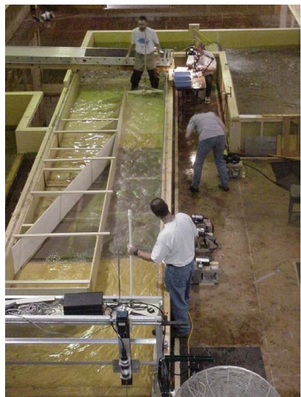
Figure 37.—Control test setup for bull trout testing with clear plastic over the screen and 4 ft/s sweeping velocity.
