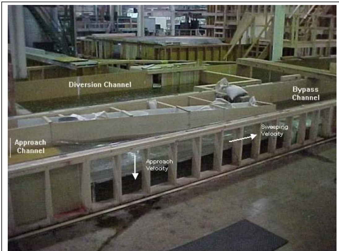
Figure 2.—Overall view of the horizontal screen model showing the flow channel designations and velocity orientations.
