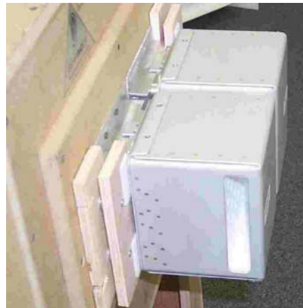
Figure 5: CGBA muffer attached to test fixture
