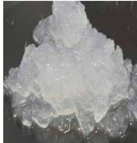
Fig. 1. Photograph of clay fraction isolated from Yucca Mountain alluvium. The clays are light yellowish, gel-like, and transparent. Field of view is ~5cm.
