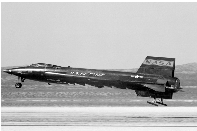
An X-15 lands on a lakebed in 1961. The X-15 was a 50-foot single-seat rocket aircraft launched from under the wing of a converted B-52 bomber. The vehicle, a precursor to the Shuttle, brushed the threshold of space.
