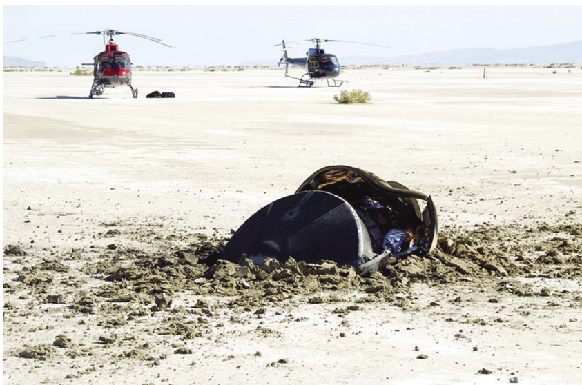
The Genesis sample-return capsule isn't buried in the ground—it's smashed. The capsule crashed near Granite Peak on a remote portion of the Utah Test and Training Range.
