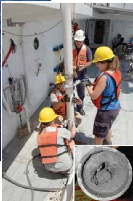
Matt Arsenault (USGS, left) and Jim Broda (WHOI) recover the Giant Gravity Corer aboard the R/V Seward Johnson after deployment of the corer into the Mona Canyon. Photograph by Uri ten Brink (USGS).
