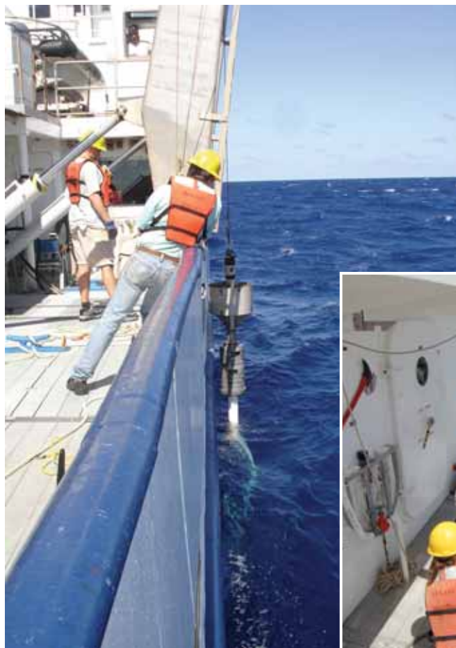
Matt Arsenault (USGS, left) and Jim Broda (WHOI) recover the Giant Gravity Corer aboard the R/V Seward Johnson after deployment of the corer into the Mona Canyon. Photograph by Uri ten Brink (USGS).
