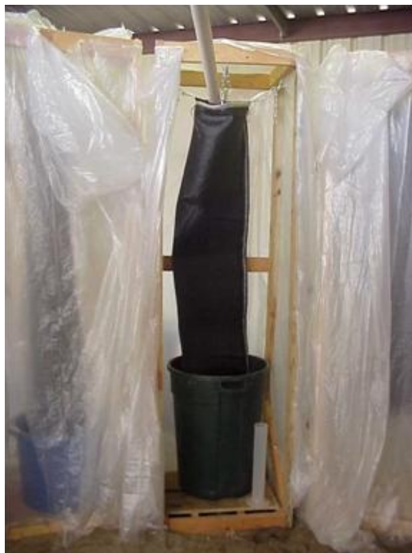
Figure 2. Geotextile bag (center) and frame used to conduct a hanging-bag test.
