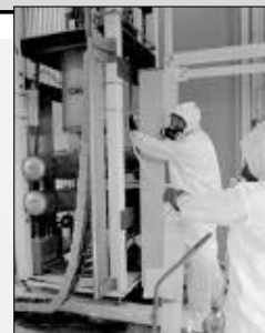
Employees from Advanced Nuclear Technology (NIS-6) perform a fuel exchange operation on the SHEBA assembly. The protective equipment, including respirators, is worn to guard against inadvertent contamination. Photo courtesy of
