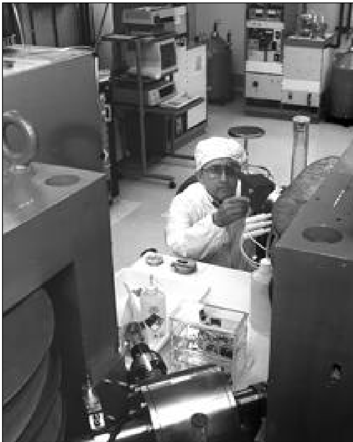
Don Rokop of Environmental Science and Waste Technology (CST-7) uses the thermal ionization mass spectrometer in the clean laboratory at TA-48 to check urine samples for plutonium. Photo by John Flower of Photo, Video, Digital Imaging (CIC-9)
