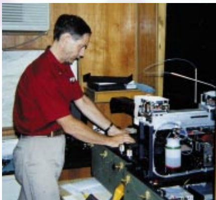
Figure 1. Ray Mariella, Jr., working with a multichambered PCR (polymerase chain reaction) unit. In the 1997 Advanced Concept Technology Demonstration, this PCR instrument proved an effective tool for field identification of the DNA in nonvirulent bioagent simulants.
