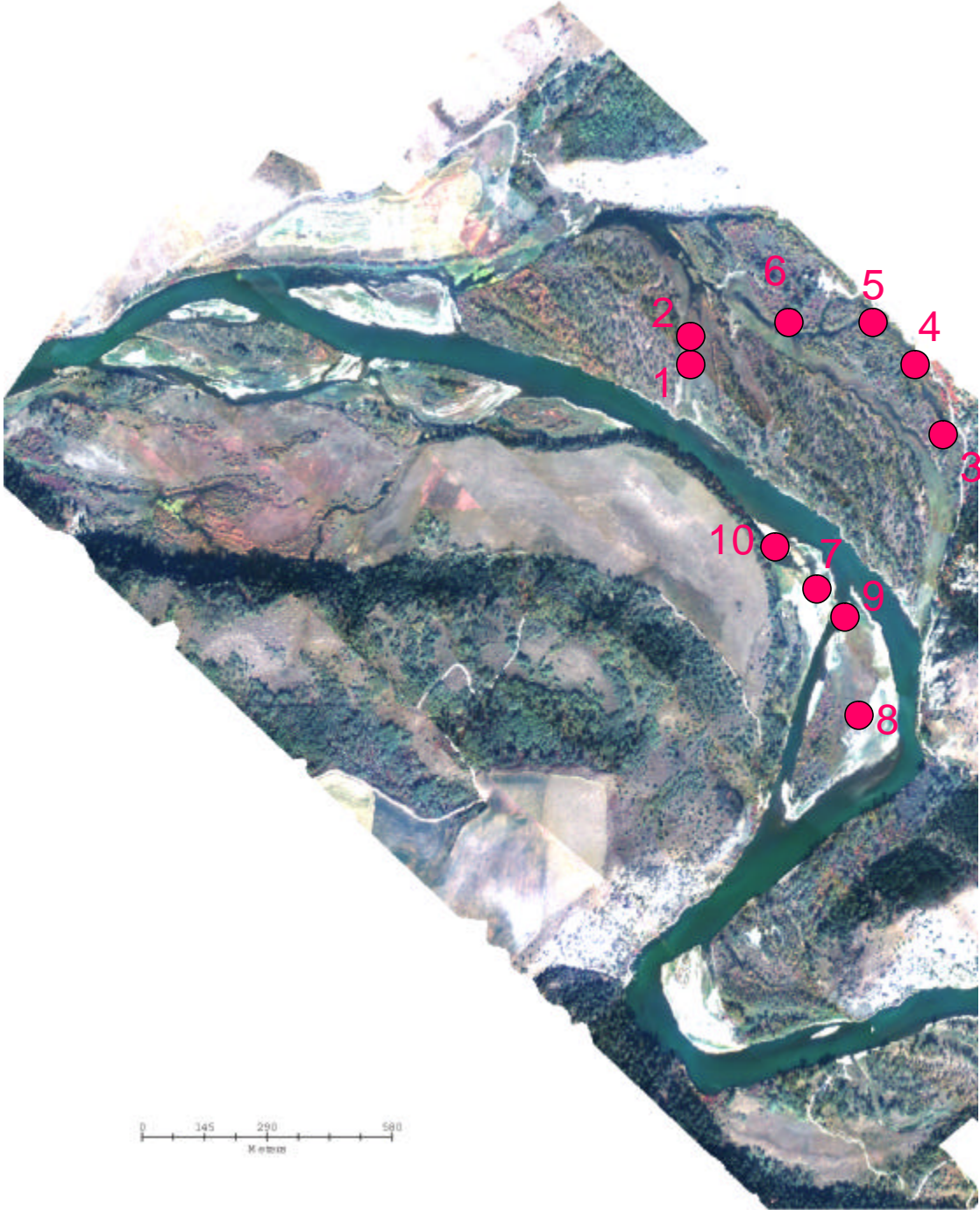
APPENDIX A Figure 13. Georectified hyperspectral image of the Fisher floodplain with locations of Temperature loggers. Temperatures were recorded every two hours for 16 months. Data are displayed in the following figures.
