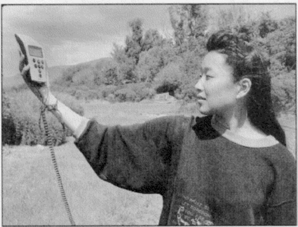
Creek Watch intern Diane Kodama demonstrates the "GPS stance." The GPS receiver must be held well away from the body to avoid blocking satellite transmissions.
