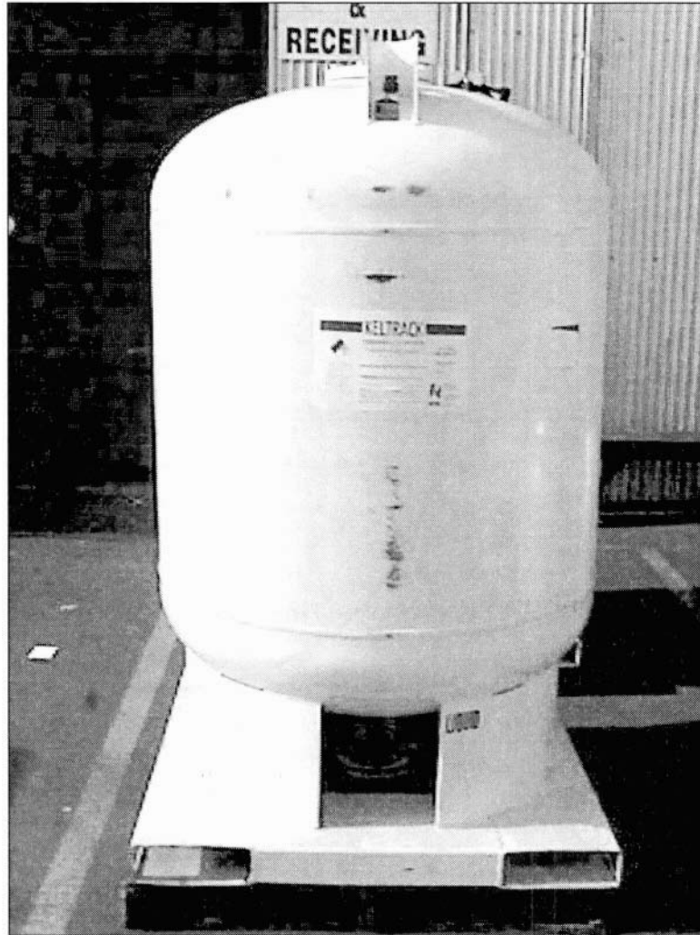
Figure 2. Pressurized Bulk Refilling Tank, CHI-TECH System, Provided by Portec Rail Products
