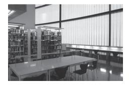
Figure 3-28. Interior view of Rapson Hall using channel glass with translucent insulation. Channel glass is used as a linear glazing system, with translucent insulation sandwiched between interlocking pieces of glass. The channel glass itself has a U-factor of 0.53, SHGC of 0.69, and VT of 0.75. The insulation improves the assembly U-factor to 0.29 and SHGC to 0.36. VT falls to 0.38. Photo: Warren Bruland
