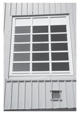
Figure 3-31. Field test of electrochromic windows at LBNL. (Left) Interior view of EC window with the lefthand window column set to fully bleached or clear and the righthand window column set to fully colored. The middle window column is set to a transmission level halfway between the two extreme states. (Right) Exterior view of EC window. Photo: Courtesy of LBNL; Photo: Roy Kaltschmidt
