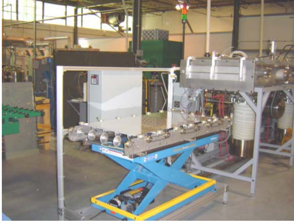
Figure 9: Photo of Automatic Unloader on Sputtering System
