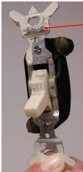
Photo 21. Mercury Containing Switch. Townsend 2004 (Ref. 28)
