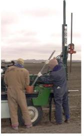
Soil water content, organic matter, organic nitrogen, pH, nitrate, and ammonium concentration are routinely determined on soil samples obtained with a hydraulic sample mounted on a pickup.
